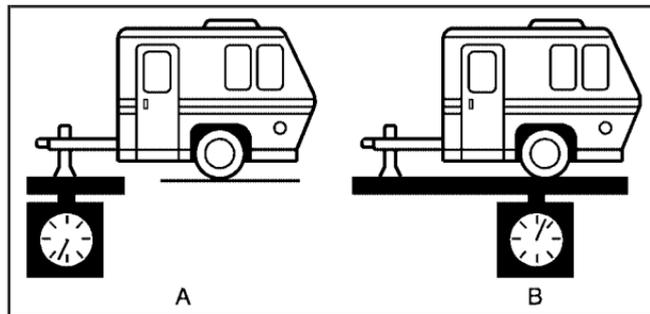
If you are using a weight-carrying hitch or a weight-distributing hitch, the trailer tongue (A) should weigh 10-15 percent of the total loaded trailer weight (B).
