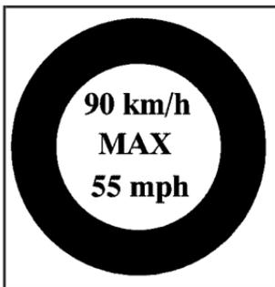
16. If the flat tire was able to inflate to the recommended inflation pressure, remove the maximum speed label from the sealant canister (B).
