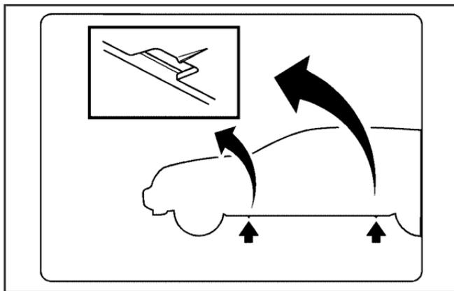
4. To identify the appropriate jacking location, find the V-shaped locating notches in the molding.
