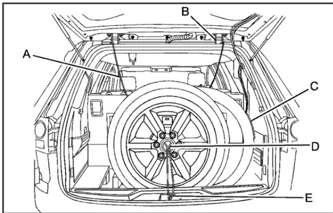
4. Hook one end of the cable onto the outside portion of the liftgate hinge opposite (B).
