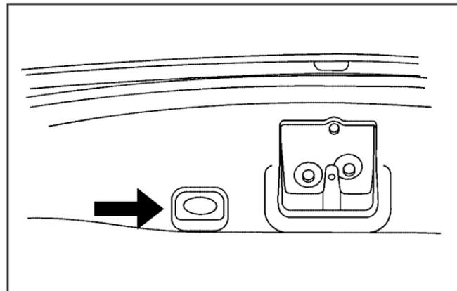
**Power Liftgate Button Near Liftgate Latch**
