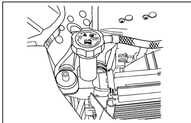
7. Start the engine and let it run until you can feel the upper radiator hose getting hot. Watch out for the engine cooling fan.
