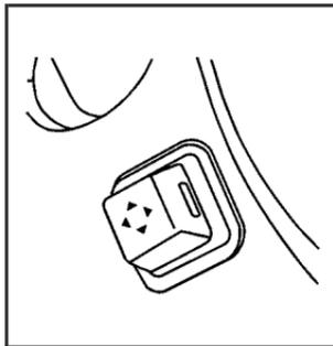
For vehicles with the power tilt wheel control, it is located on the left side of the steering column.
