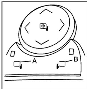
If your vehicle is equipped with outside power mirrors, the controls are located on the driver door armrest.
