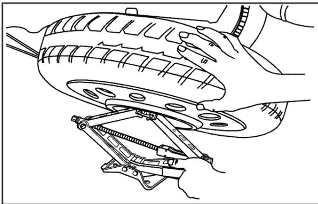
8. Disconnect the lug wrench from the jack and carefully remove the jack. Use one hand to push against the spare tire while firmly pulling the jack out from under the spare tire with the other hand.
