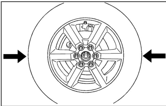
The tire valve stem must be positioned between the 3 and 9 o'clock positions.
