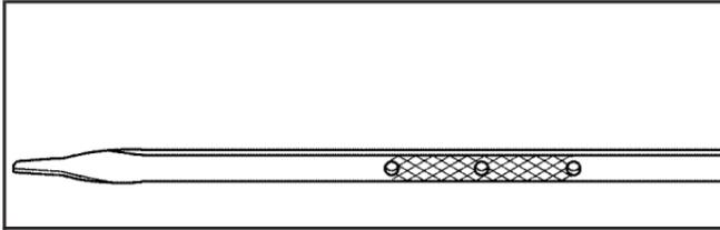
If the oil is below the cross-hatched area at the tip of the dipstick, add at least one quart/liter of the recommended oil. This section explains what kind of oil to use. For engine oil crankcase capacity, see *Capacities and Specifications on page 5-120*.
